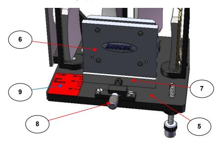
Fig 2. Translation Stage with Fitted ATR Crystal and Solids Holder Assembly
