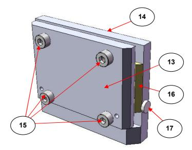
Fig 3. Solids Holder Assembly with ATR Crystal
