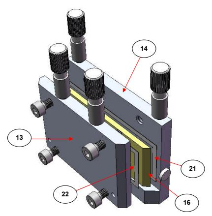
Fig 7. ATR Crystal with Gaskets for Sample Cavities as Positioned in the Liquids Holder
