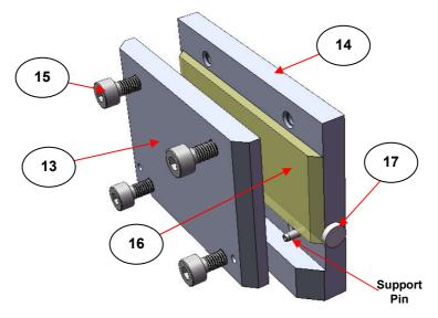
Fig 4. ATR Crystal as Positioned in the Solids Holder
