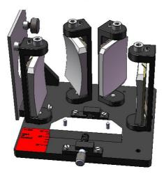
• 1 Solids sample holder P/N GS11001 with a ZnSe crystal P/N GS11014 fitted and mounted for use.
